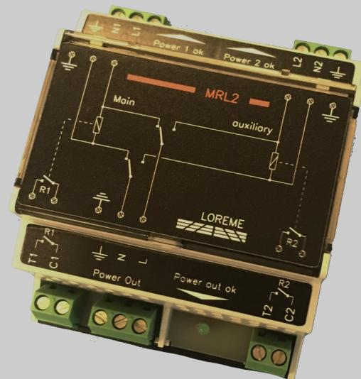
The redundancy module provide an effective protection against the failure of AC power supplies. Through de-coupling of two power supplies, the failure of one of them has no effect on output, the other taking automatically its function without interruption.
